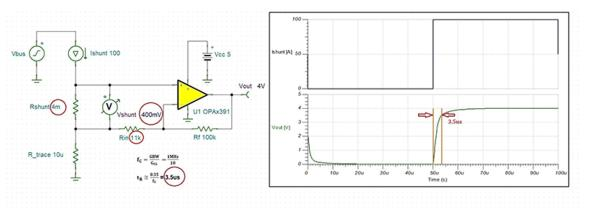
Figure 4. Rise time of the OPA391 low-side current shunt signal for G = 10
