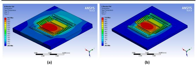
Figure 4-2. Simulation Results of Temperature Distribution for ts-QFN 12x12 Package with (a) Gel TIM and (b) Pad TIM
