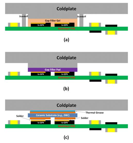
Figure 3-3. Thermal Management Solutions for ts-QFN 12x12 Package with Coldplate Using (a) Gap Filler Gel, (b) Gap Filler Pad, and (c) Thermal Grease/DBC Substrate
