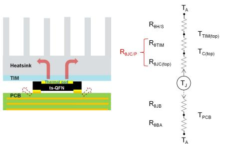
Figure 3-1. Top-Side Cooling Configuration and Thermal Resistance (R $_{\theta}$ ) Model
