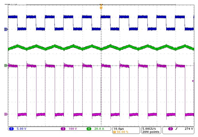
Figure 6-4. Buck Operation at 6 kW with Coldplate
