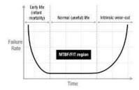
TI's MTBF/FIT estimator search tool allows you to find generic data based on technology groupings to estimate these typical questions and shows conditions under which the rates were derived.
