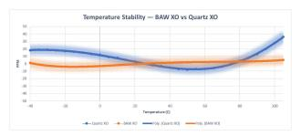
Figure 4. Temperature Stability Comparison of BAW Oscillator and Quartz
