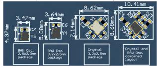
Figure 2. PCB Footprint Comparison of BAW Oscillator and Crystal
