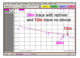
a limiting redriver can launch a large swing signal with de-emphasis and potentially make the channel compliant.
