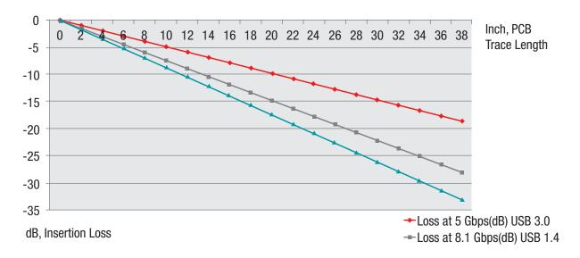
Figure 3. USB Type-C USB/DisplayPort insertion loss profile for 4-mil-wide FR-4 PCB trace loss.
