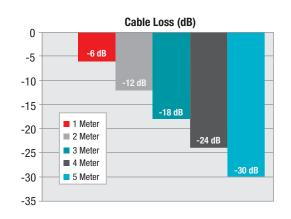
Figure 2. USB Type-C cable loss profiles for 10 Gbps signals.
