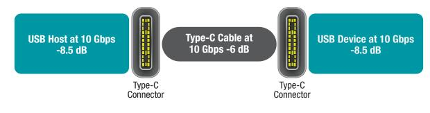
Figure 5. USB 3.1 Gen 2 at 10Gbps USB Type-C channel-loss budget.
