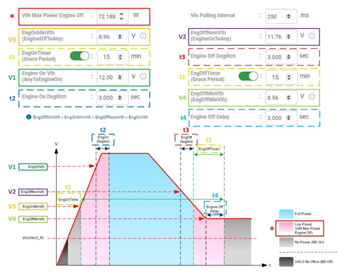
Figure 4-6. Engine On or Off GUI Entry Example
