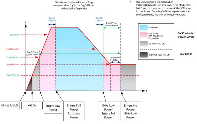
Figure 4-5. VIN Level and Engine On or Off Power Transition
