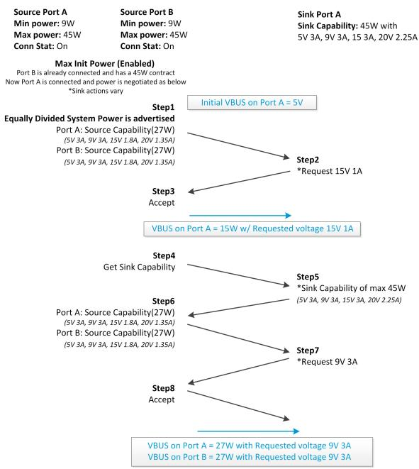
Figure 5-12. Hybrid Mode Negotiation Flow - Scenario 2
