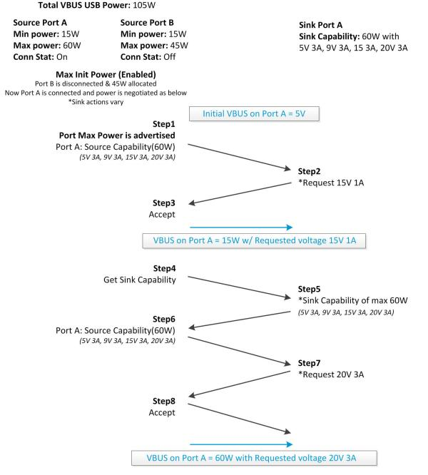
Figure 5-1. Assured Capacity Policy Negotiation Flow - Port A Connected
