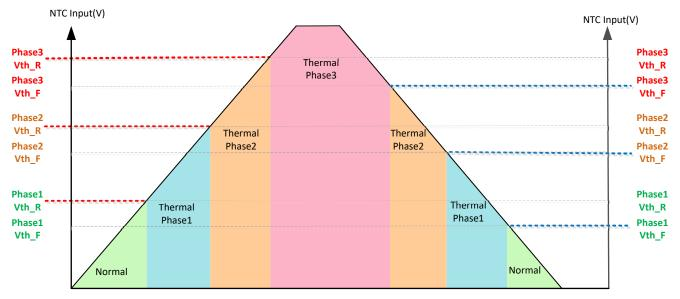
Figure 4-1. NTC Input Voltage Threshold and Thermal Phase
