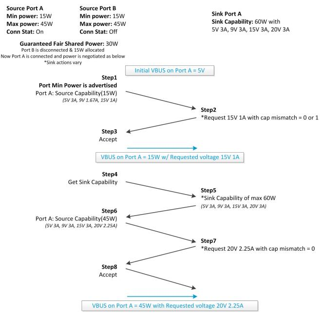
Figure 5-3. FSP Negotiation Flow - Scenario 1
