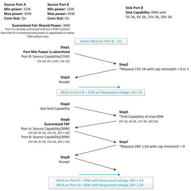
Figure 5-4. FSP Negotiation Flow - Scenario 2
