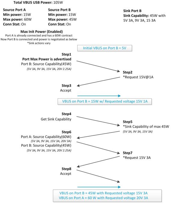
Figure 5-2. Assured Capacity Policy Negotiation Flow - Port B Connected
