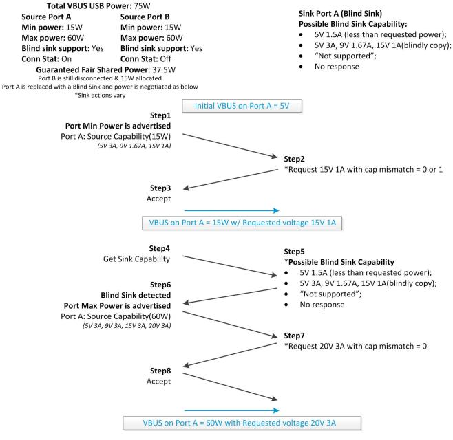
Figure 5-6. FSP Negotiation Flow with Blind Sink Support – Scenario 2
