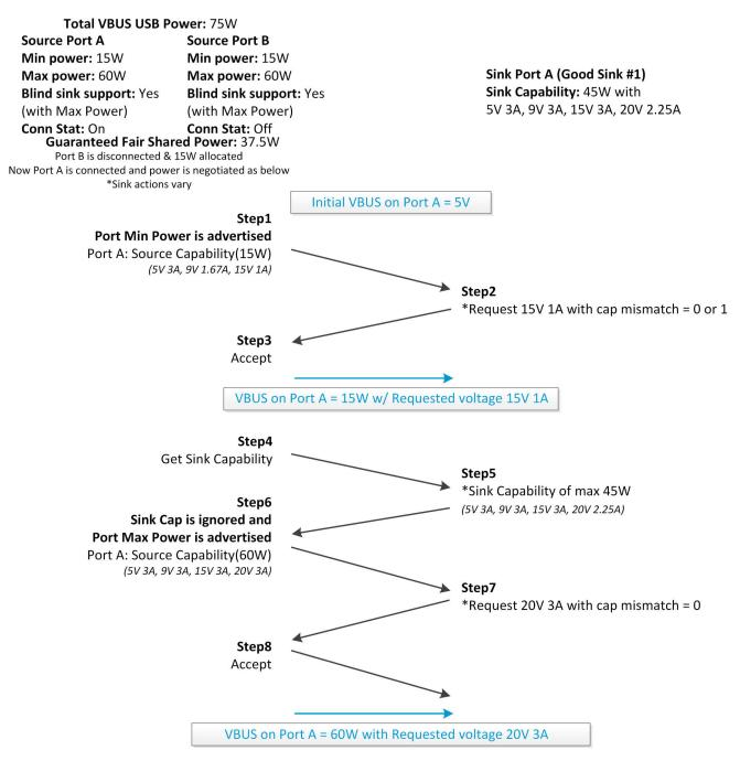
Figure 5-8. FSP Negotiation with Blind Sink Support & Max Power - Scenario 1
