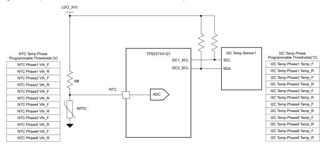
Figure 4-4. I2C Temp Sensor and Thermistor Configuration Example
