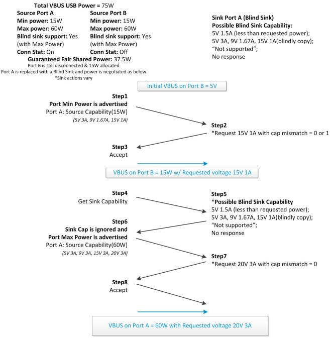
Figure 5-9. FSP Negotiation with Blind Sink Support & Max Power - Scenario 2
